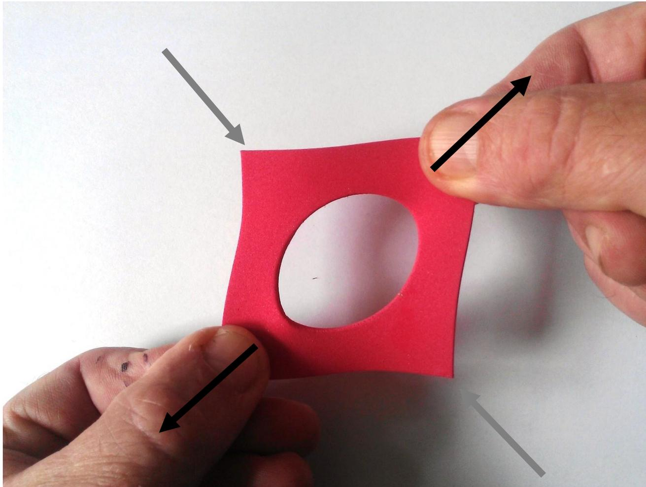
This is a piece of soft cellular rubber with a circular hole. Pulling the opposite corners, you see the effect of the force (or of the tension) on the deformation of the hole.
